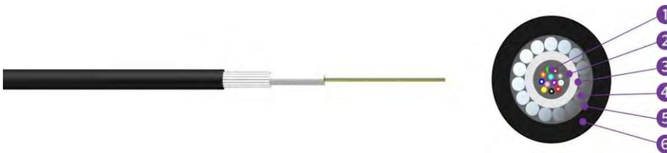
1, Fibers    2, Tube Filling Compound    3, Loose Tube    4, Steel wire    5, Cabling compound    6, PE Sheath
