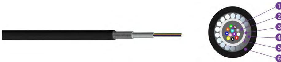
1, Fibers 2, Tube Filling Compound 3, Loose Tube 4, FRP wire 5, Water Blocking Yarn 6, PE Sheath
