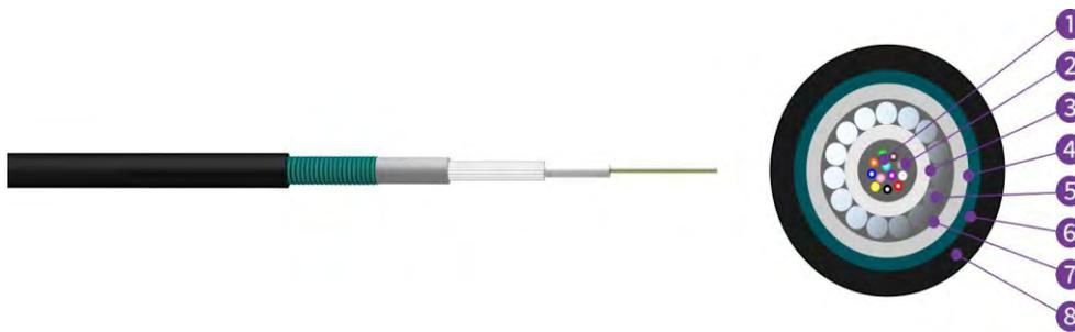
1, Fibers 2, Tube Filling Compound 3, Loose Tube 4, PE Inner sheath 5, Steel wire 6, PSP 7, Cabling compound 8, PE Sheath
