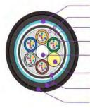
Armor Water Blocking Material Moisture-proof Loose Tube Thermoplastic Central Strength Member GFRP Filler Elements Thermoplastic rods Sheath Black PE Anti-termite Sheath Nylon
