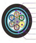
Armor Loose Tube Thermoplastic Water Blocking Material Optical Fiber Central Strength Member Phosphate steel wire Filler Elements Thermoplastic rods Anti-Rodent Armor Sheath Black PE
