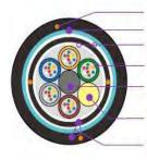
Ripcord Armor Water Blocking Tape Loose Tube Thermoplastic Central Strength Member GFRP Filler Elements Thermoplastic rods Sheath Black PE
