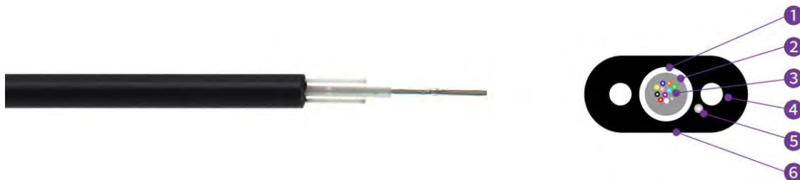
1, Fibre 2, Strength Member 3, Sheath 4, Tube Filling Compound 5, Water Blocking Yarn 6, Loose Tube
