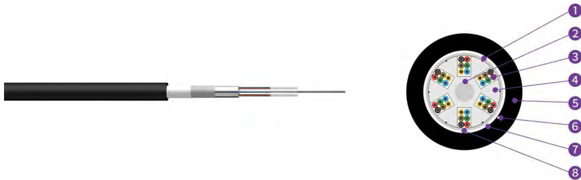
1, Rib Mark 2, Strength Member 3, Tight Buffered Fibre 4, Slot 5,Sheath 6,Ripcord 7,APL 8,Water Blocking Tape
