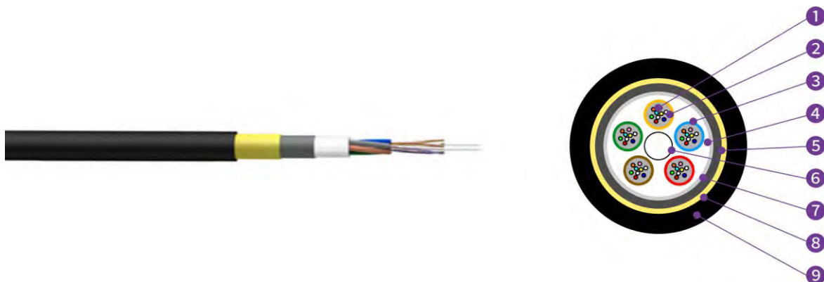
1, Fibers 2, Tube Filling Compound 3 Loose Tube with Gel 4, Cable Filling Compound 5, PE Inner Sheath 6, CSM 7, Aluminum Tape (APL) 8, Aramid Yarns 9, PE Outer sheath
