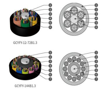
1, PE Sheath 2, Water Blocking Yarn 3, Loose Tube 4, Strength Member 5, Fibre 6, Tube Filling Compound 7, PE Layer
