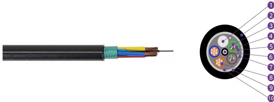
1,Filler 2,PE Sheath 3,Fibre 4,Tube Filling Compound 5,Loose Tube 6,Strength Member 7,Ripcord
