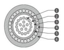
1, Fibers 2, 3, Tube Filling Compound 4, FRP wire 5, Waterr Blocking Yarn 6, PE Sheath
